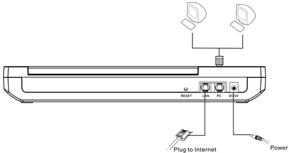
Connect the network cable linking the network to the LAN port, and the configuration PC or other shared PC in the network to the PC port. The LAN port can be connected to the ADSL Modem, Switch or Ethernet private lines. The SMB32 supports fixed IP and IP acquisition through DHCP and PPPoE.
